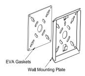
4. Lift the fixture and arrange the anti-falling wire rope to avoid being exposed to the fixture or obstructing the installation. Fasten the fixture to the wall mounting plate, make sure that the wires are not pulled or pinched. Tighten the two M6\*20-SS screws in step 1
