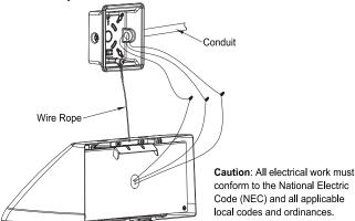
4. Lift the fixture and arrange the anti-falling wire rope to avoid being exposed to the fixture or obstructing the installation. Fasten the fixture to the wall mounting box, make sure that the wires are not pulled or pinched. Tighten the two M6\*20-SS screws in step 1.
