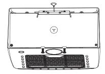
2. Knock off one of blind hole in the four sides of the mounting box to guide the wiring. Stick EVA gaskets on the back of the wall mounting box properly, which is very important for water proof. Fix the wall mounting box on the junction box according to the arrow pointing upwards.
