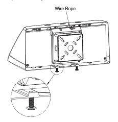
Note: To ensure waterproof seal, apply weatherproof silicone sealantaround the edge of the wall mounting box and /or junction box.
