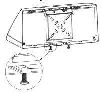
3. Hang the fixture on the wall mounting plate with a wire rope, and pay attention to protect the surface of the fixture during installation to prevent scratches and damage to the surface. Ensure the line voltage at the fixture is correct, make all necessary wiring connections, and push all the wires and wire nuts into the i-box
