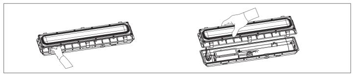
1. Unfasten the latches and separate the led module and the power housing.
