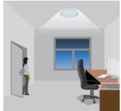
When natural lighting conditions fall below a selected threshold, the motion sensor turns on the fixture when motion is detected.
