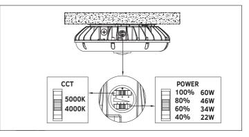
**NOTE:** Power values indicated in diagram are based on tested values and may slightly vary.
