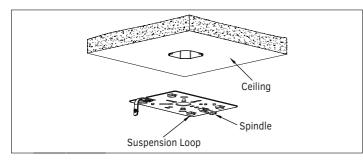
Connect the clip of the fixture to the spindle of the mounting plate to ensure the fixture will not slip and fall. Complete wiring using the wiring diagram, then push the pressing plate into the suspension loop on the mounting plate.
