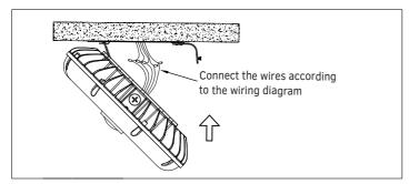
Reattach the mounting plate to the fixture using the previously removed M4 Screws.
