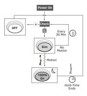
Settings In This Demonstration: Hold-Time: 30 Minutes Setpoint On: 50 Lux Setpoint Off: 300 Lux Stand-By Dimming Level: 10% Stand-By Period:  $+\infty$
