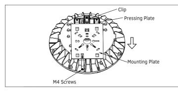
Attach the mounting plate to the ceiling using M16 Expansion Bolts or M6 stainless steel screws with plastic anchors (not included).
