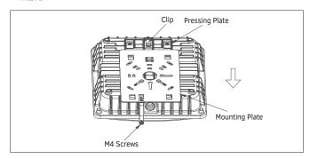
3. Connect the clip of the fixture to the spindle of the mounting plate to ensure the fixture will not slip and fall. Complete wiring using the wiring diagram, then push the pressing plate into the suspension loop on the mounting plate.
