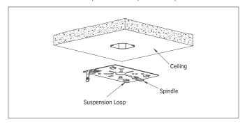
4. Reattach the mounting plate to the fixture using the previously removed M4 Screws
