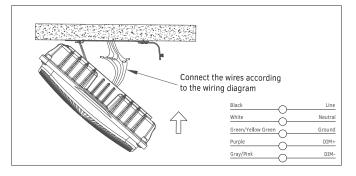
2. Attach the mounting plate to the ceiling using M16 Expansion Bolts or M6 stainless steel screws with plastic anchors (not included).
