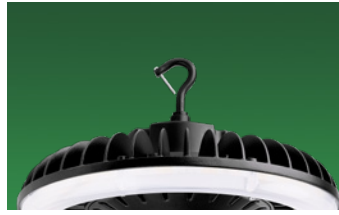
HOOK MOUNT (180W, 215W) Included M10 hook mount features an anti-shedding screw for added security.
