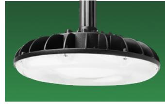
PENDANT MOUNT A 3/4" conduit entry point ensures easy pendant installation. Conduit adaptor is required for pendant mounting 180W and 215W models (as shown below under Accessories).
