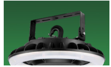
ADJUSTABLE SURFACE MOUNTING BRACKET Allows precise aiming of the fixture to 0°, 30°, 60°, 90°, 120°, 150°, or 180° - not available for 180W or 215W.
