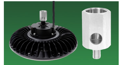
CONDUIT ADAPTOR Allows conduit pendant mounting for 180W and 215W models. The adaptor screws into the M10 hole on the top of the fixture and includes a 3/4" thread for a standard 3/4" conduit. Left: installed view of conduit adaptor. Right: uninstalled view of conduit adaptor.
