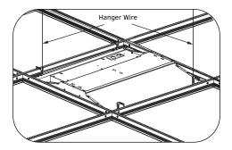
3. Use a hanger wire to secure fixture to the grid in compliance with state and local codes. Screws and hanger wires are not included with fixture.
