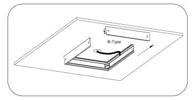
3. Remove one of the B-Type frames by pushing in the tabs from the connectors and pulling the frame out.
