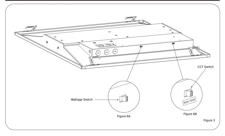
The end user may adjust the CCT and lumen output using two DIP switches integrated into the driver. Each DIP switch has 3 settings (left, middle, right) respectively corresponding to 3 CCT and 3 wattage options.
