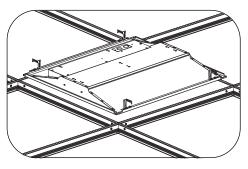
2. Install the fixture into the T-bar ceiling grid. Ensure that each fixture fits snugly into the ceiling grid and all fixtures are oriented in the same direction.
