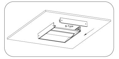
5. Replace the B-Type frame into the slot, ensuring it is locked in place by the plastic corner connectors.
