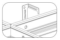
1. Locate desired fixture location in ceiling grid and remove the existing ceiling panel at chosen location. Also remove adjacent ceiling panel to allow for wiring access from above. Bend the clips on the sides of the fixture 90° to engage with the T-bar support grid.
