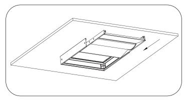
${\bf 4}.$  Make wiring connections to the main power according to local code and insert the LED Panel into the frame.
