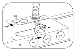
4. Remove screw on driver wiring chamber, slide cover to the side, and remove cover. Set the screw and cover aside to be reinstalled later. Remove appropriate 1/2" knockout(s) to allow for replace the adjacent ceiling panel that was entry of supply wiring into the wiring chamber.
