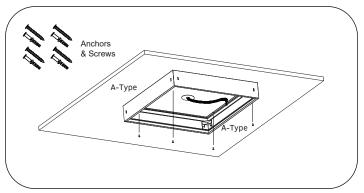
2. Using the square frame as a positioning guide, place the frame with screw holes facing up and mark their locations, then use the anchors and screws to secure the frame to the ceiling. Only the A-Type frames have screw holes, which are located closer to the center of the frame.
