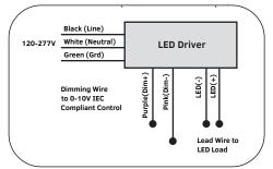
5. Follow the wiring diagram for the specific model you are installing. Replace the electrical enclosure cover and tighten the screws, then removed in Step 1.
