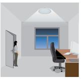
When natural lighting conditions fall below a selected threshold, the motion sensor turns on the fixture when motion is detected.
