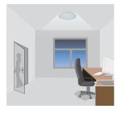
After sensor hold time elapses, the motion sensor dims the fixture to the stand-by light level if the natural light conditions are below the selected threshold.
