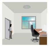
When natural lighting conditions are sufficient, the motion sensor does not turn on the fixture even when motion is detected.
