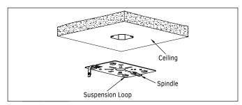
3. Connect the clip of the fixture to the spindle of the mounting plate to ensure the fixture will not slip and fall. Complete wiring using the wiring diagram, then push the pressing plate into the suspension loop on the mounting plate.
