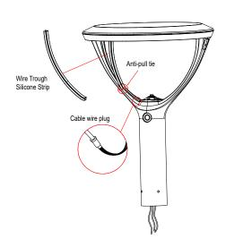
Step 4: Connect the mains power supply, assemble the lamp body, and tighten 4 pcs of M8\*16 set screws to complete the installation.
