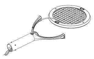
Step 2: Assemble the support arm with the lamp body and screw with 4 pcs of PM5-20 screws; assemble the side cover and tighten the 2 pcs PM3\*8 screws. (Tool: Phillips screwdriver).
