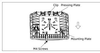
3. Connect the clip on the fixture to the spindle of the mounting plate to ensure the fixture will not slip and fall. Connect the line voltage to the fixture wires, following the wiring diagram. Push the pressing plate into the suspension loop on the mounting plate.
