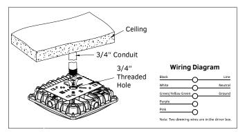
2. Attach the mounting plate to the ceiling using screws up to M5 (not included).
