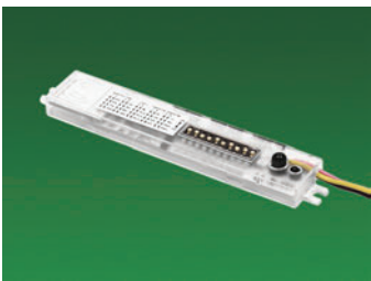
MICROWAVE MOTION SENSOR Optional field-installed microwave multi-level motion sensor detects occupancy in an area for additional energy savings.
